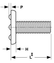
‡Length of weld studs is measured from the welding surface of the head to the end of the shank, excluding the projections.
